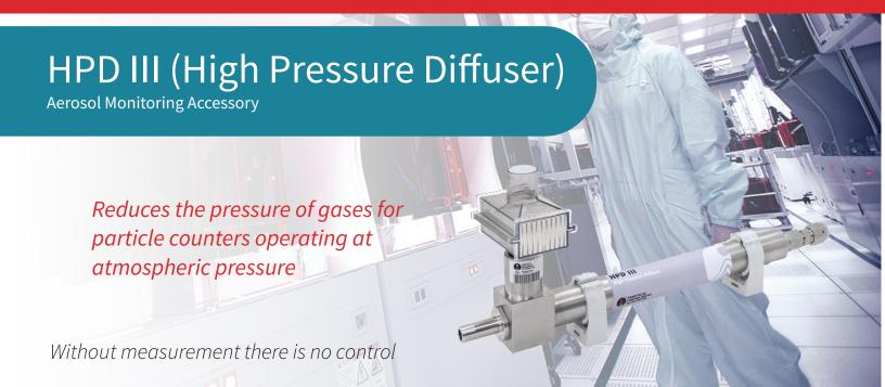
The HPD III reduces the pressure of high purity, high pressure gas to near atmospheric pressures to allow for accurate sampling of aerosol particle size channels of ≥ 0.2 μm by PMS particle counters. The HPD works by diffusing some of the gas out of the system, allowing the particle counter's flow-metering system to function as designed. The PMS particle counters that the HPD III is compatible with includes AirNet, IsoAir, Lasair Pro, and Lasair III.
